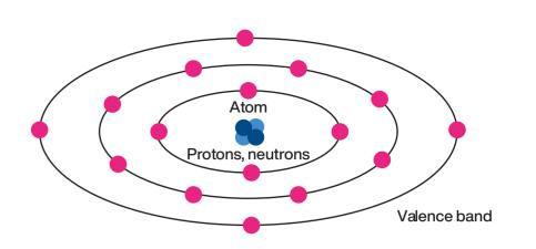
Bandgap = 0 or very small: Conductor, such as copper wire. Valence and conduction bands overlap Bandgap < 2 eV: Conventional silicon semiconductors, such as a transistor or diode Bandgap > 2 eV: WBG material semiconductors Bandgap > 4 eV: Insulator
